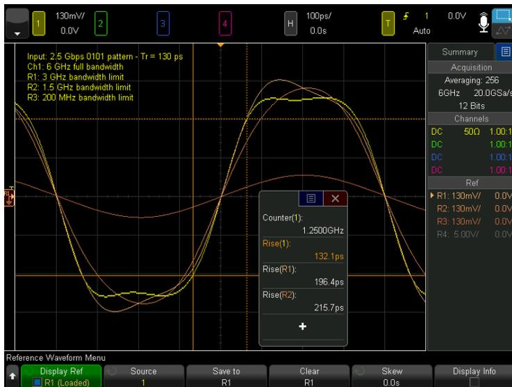
Figure 51. Reference waveforms.
