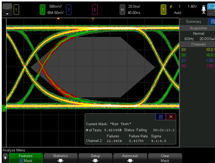
Figure 41. Mask testing of serial data.
