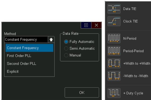
**Figure 18.** Clock recovery menu and jitter measurement menu.
