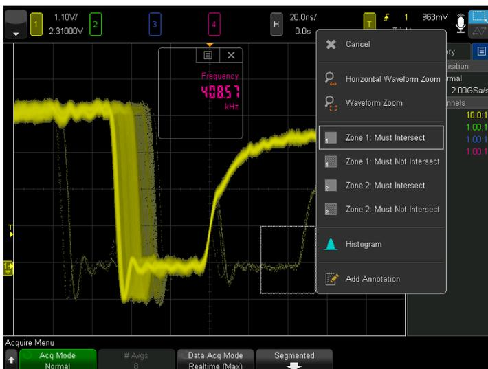
**Figure 11.** Draw a zone (box) around the anomaly.
