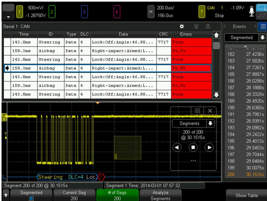
Figure 25. Segmented memory + serial bus decode + zone trigger.
