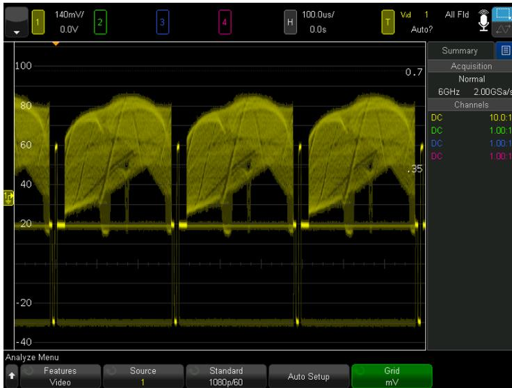
Figure 45. Triggering on a 1080p/60 signal.
