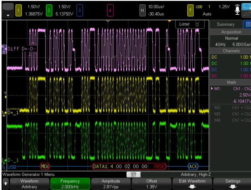
Figure 29. Dual-channel generator generating a differential signal.
